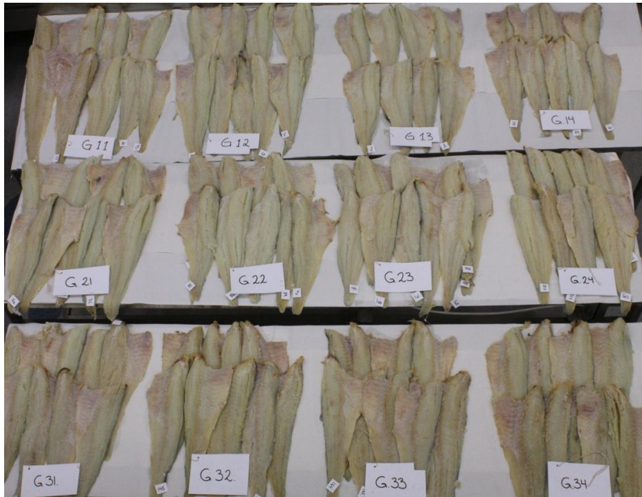
Figure 3.39. Heavy salted fillets after five months of chilled storage (N=9). G11-G14 injected and pickle salted, G21-G24 injected and brined, G31-G34 pickle salted 1:5. Increasing phosphate levels moving to the right.
